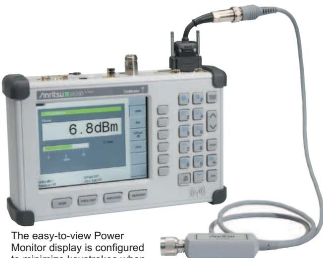
The easy-to-view Power Monitor display is configured to minimize keystrokes when testing in the field.
