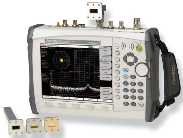
*Precision waveguide-to-coaxial adapters enable VNA Master to conduct calibration and measurement in a variety of popular waveguide flange types.*
