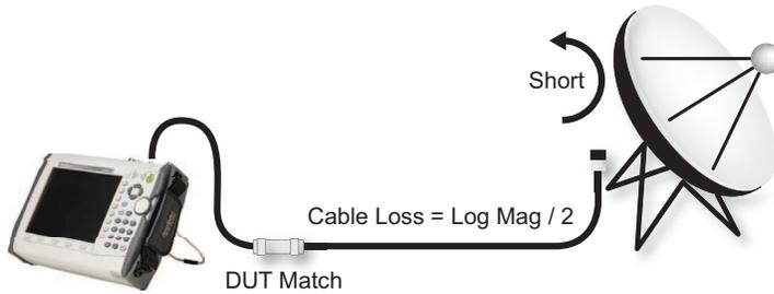
This illustration shows the popular setup for conducting round-trip cable loss measurements. This technique involves using a short at the far end and measuring reflections at the near end of the cable. The test signal traverses the cable twice so cable loss is one-half of the reflection measurement.
