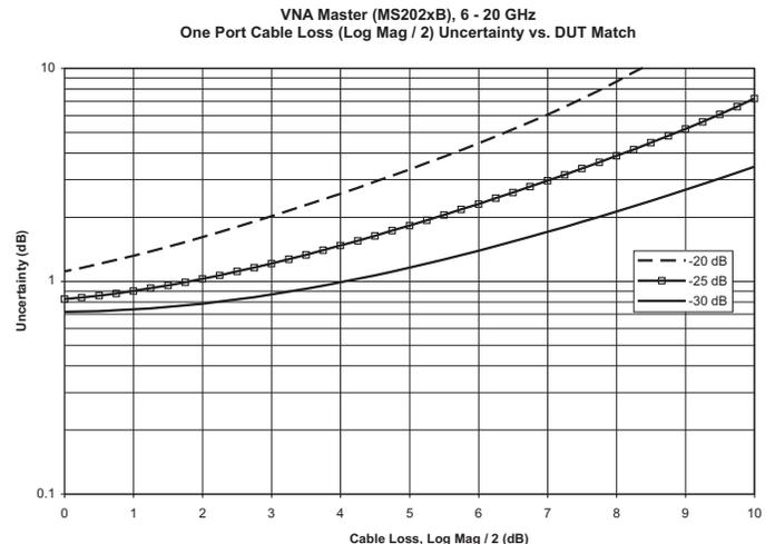
These uncertainty curves show how frequency range, DUT Match, and cable loss impact worst-case uncertainty of round-trip cable loss measurements. The uncertainty curves, separated by frequency range, are shown for DUT Match conditions of 20, 25, and 30 dB. For DUT Match of 30 dB and cable loss of 4-5 dB (reflection measurement of 8-10 dB) the worst-case uncertainties are approximately  $\pm 1$  dB.
