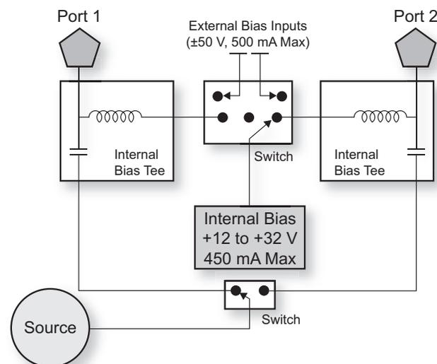
The VNA Master offers optional integrated bias tee for supplying DC plus RF to the DUT as shown in this simplified block diagram. Connectivity is also provided for external supply (instead of internal) to preserve battery consumption.
