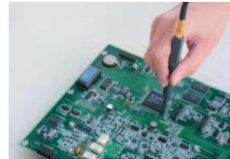
Typical applications of this magnetic field probe are evaluation of the effectiveness of a bypass capacitor located near the power supply terminal of an IC or evaluation of the microstrip layout on a PCB. Due to the probe's high spatial resolution (approximately 0.25 mm), it is not affected by adjacent patterns.
