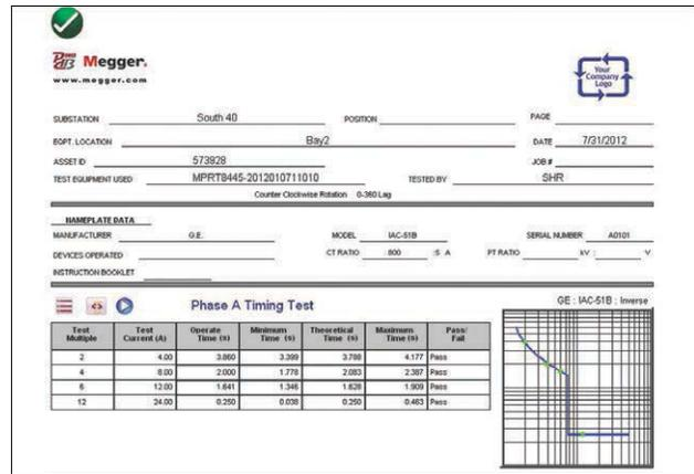
Figure 5. Test Report G.E. IACSIB Timing Test
